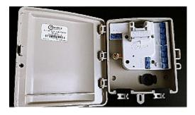
The Dual All-In-One NID is the complete solution for ease and savings of installation of Bonded VDSL2 service. The All-In-One seals two GDT primary protectors with IDC inputs, two VDSL2 splitters, two IDC outputs for modem 1 & 2 and 7 IDCs for POTS for Line 1 and 1 IDC for POTS Line 2 altogether. The Dual All-In-One is housed in its own outdoor rated enclosure.
