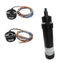
The CNI Load Coil is placed along a telephone line to compensate for the losses in signal over long distances. The load coil induces an electrical current via magnetic fields to compensate for lost signal power. Both 66mH & 88mH are available and designed to moderate the loss in signals, or attenuation, or minimize it at high voice frequencies in telephone lines.
