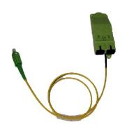
The Optical Splitter's role is to split the signal evenly from a single fiber into two fibers. The "ln" side consists of a 2 Ft (0.6m), 2.0mm yellow pigtail, with a terminated SC/APC connector. The "Out" side consists of two female SC/APC adapters.
