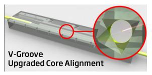
Improved Performance. Even Lower Loss now. A Flat Cleave Technique with a Reflectance Performance of Grade 1 specifications > 60dB. Average values: IL 0.03DB, RL 63dB, using KeyCleave®. Upgraded Core Alignment. In the strictest sense, KeyQuick® Mechanical Splice is a permanent connection made between two optical bres for an indenite period of time without movement. MS201 is viable for analog signal transmission. For quicker connections, home drops and network applications.
