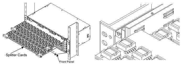
The 4192 shelf is equipped with a hinged Front Panel that is held in place by two 6-32 captive screws. Carefully unscrew the Front Panel's captive screws (either by hand or with a ¼" [6.5mm] slotted screwdriver). Rotate the Front Panel down and out of the way.
