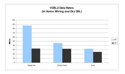
In the daisy chain configuration, there is a 47% reduction in downstream and 1% reduction upstream.
