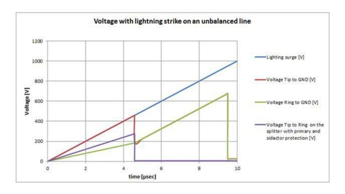
This figure illustrates the faster response time solid-state sidactor devices have to impulse strikes than GDTs. The quicker response time results in better protection of the CPE equipment and a reduction in damaged field units.
